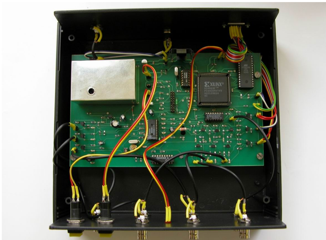
Fig.13 Complete produced PAL flexible analogue electronic images generator
